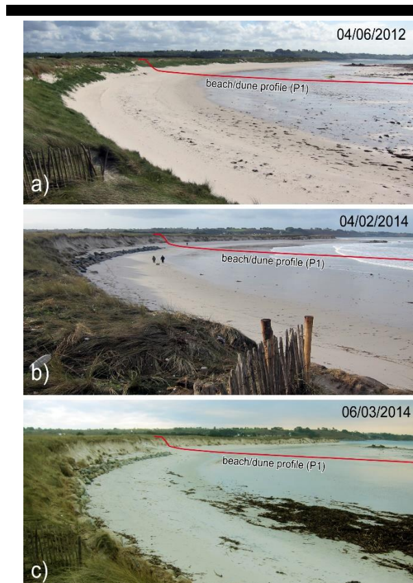
Figure 9. Shoreline retreat on Vougot beach during the stormy winter of 2013-2014. Pre-storm situation (a), post-storm situation (b) and after the storm of February 1-2, 2014 (c).
