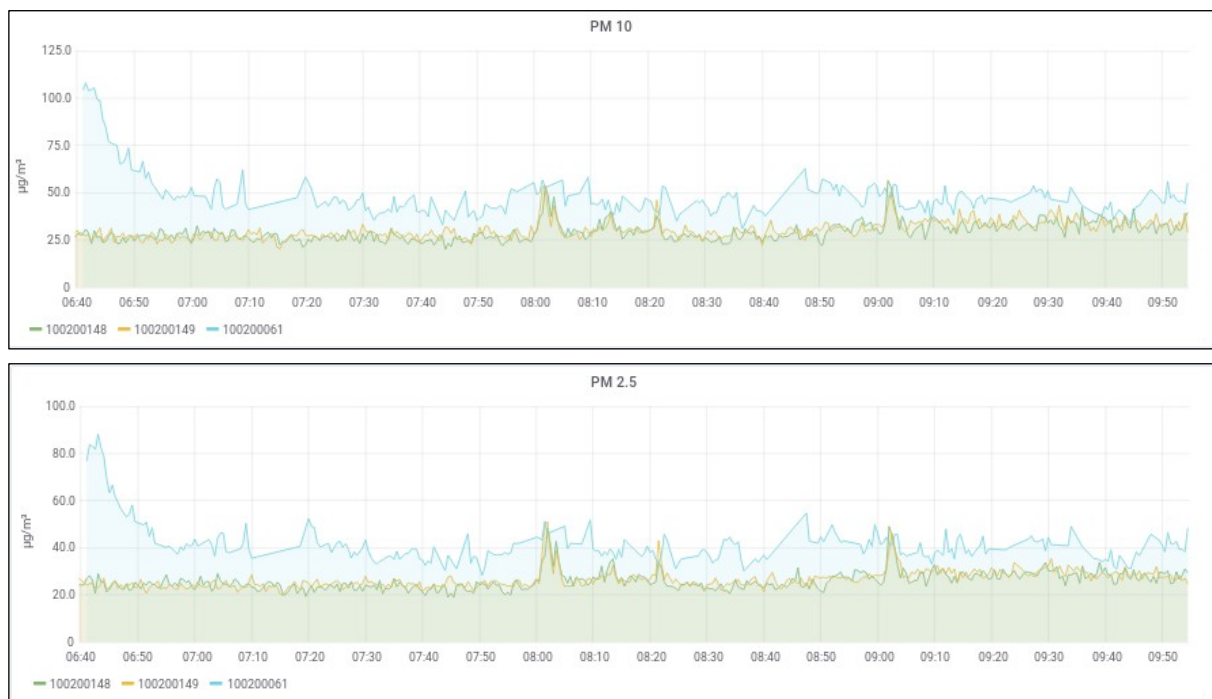
Figure 8: PM10 and PM2.5 concentration time-series (in µg/m 3 ) on 8 April 2019 between 6:40 am and 9:50 am local time. The blue line indicates measurements on the moving bus. Yellow and green lines correspond to measurements at the fixed site of Laennec.
